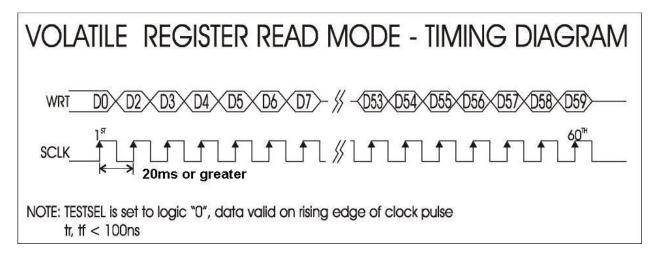
Volatile register Readout - Timing Diagram
